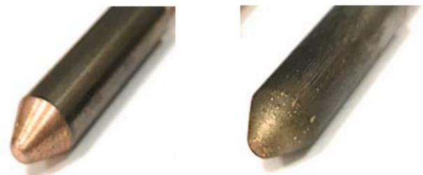
a) Before arc experiment      b) After arc experiment
